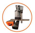
CAUTION: Electro-magnets of any machine used with the OverReach should be contained on the plate area at all times in use & must not over-hang
