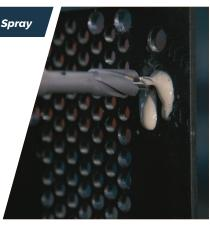
SpeedLube™ is a high performance foaming lubricant suitable for a wide variety of metal drilling applications across a range of materials including stainless steel.
